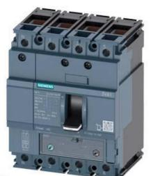
CIRCUIT BREAKER 3VA1 IEC FRAME 160 BREAKING CAPACITY CLASS N ICU=25KA @ 415 V 4-POLE, LINE PROTECTION TM240, ATAM, IN=160A OVERLOAD PROTECTION IR=112A ...160A SHORT CIRCUIT PROTECTION II=5...10 X IN NEUTRAL PROTECTION 50% CABLE CONNECTION
