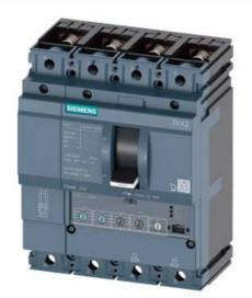
CIRCUIT BREAKER 3VA2 IEC FRAME 250 BREAKING CAPACITY CLASS C ICU=110KA @ 415 V 4POLE, LINE PROTECTION ETU330, LIG, IN=160A OVERLOAD PROTECTION IR=64A ...160A SHORT CIRCUIT PROTECTION II=1,5...12 X IN NEUTRAL PROTECTION ADJUSTABLE(OFF,50%,100%) GROUNDFAULTPROTECTION IG=0,2... 1 X IN, TG=0,1/0,3MS BUSBAR CONNECTION
