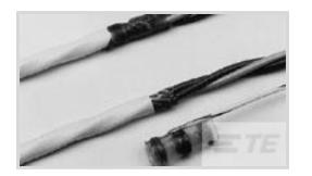
Operating Temperature (Max): 125 °C Expanded Inside Diameter (Min): 2.67 mm [.105 in ] Recovered Inside Diameter (Max): 1.27 mm [.05 in ] Pre-Installed Lead: No Wire Size: .34 mm<sup>2</sup>
