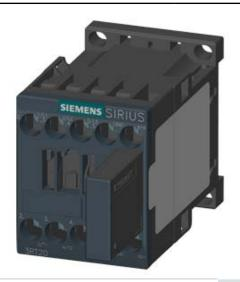
COUPLING RELAY, AC-3, 4KW/400V, 1NO, DC 24V, 0.85...1.85\*US, W. PLUGGED-ON VARISTOR 3-POLE SZ S00, SCREW TERMINAL
