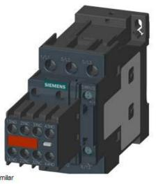
CONTACTOR, AC-3, 15KW/400V, 2NO+2NC, 24 V DC, W. INSERTED VARISTOR 3-POLE, SIZE S0 SCREW CONNECTION AUX. SWITCH PERMANENTLY MOUNTED
