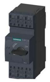
CIRCUIT-BREAKER SZ S0, FOR MOTOR PROTECTION, CLASS 10, A-RELEASE 11...16A, N-RELEASE 208A, SPRING-L. CONNECTION, STANDARD SW. CAPACITY,
