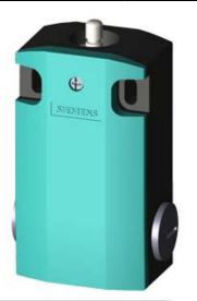
SIRIUS POSITION SWITCH, . METAL, 56MM, INCREASED CORROSION PROTECTION, DEVICE CONNECTION 3X (M20X1.5) 1NO/1NC QUICK-ACT.CONTACTS FUNCTIONAL AT -40 DEGREES, SHOCK-AND VIBRATION TEST ACC.TO EN61373, CATEGORY 1B
