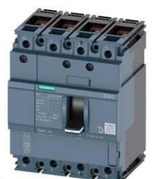
CIRCUIT BREAKER 3VA1 IEC FRAME 160 BREAKING CAPACITY CLASS H ICU=70KA @ 415 V 4-POLE, LINE PROTECTION TM210, FTFM, IN=100A OVERLOAD PROTECTION IR=100A FIXED SHORT CIRCUIT PROTECTION II=10 X IN NEUTRAL UNPROTECTED BUSBAR CONNECTION
