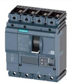
CIRCUIT BREAKER 3VA2 IEC FRAME 100 BREAKING CAPACITY CLASS M ICU=55KA @ 415 V 4POLE, LINE PROTECTION ETU850, LSI, IN=63A OVERLOAD PROTECTION IR=25A ...63A SHORT CIRCUIT PROTECTION ISD=0,6..10X IN, II=1,5..12X IN NEUTRAL PROTECTION ADJUSTABLE (OFF, UPTO 160%) BUSBAR CONNECTION
