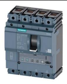
CIRCUIT BREAKER 3VA2 IEC FRAME 160 BREAKING CAPACITY CLASS L ICU=150KA @ 415 V 4POLE, LINE PROTECTION ETU330, LIG, IN=160A OVERLOAD PROTECTION IR=64A ...160A SHORT CIRCUIT PROTECTION II=1,5...10 X IN NEUTRAL PROTECTION ADJUSTABLE(OFF,50%,100%) GROUNDFAULTPROTECTION IG=0,2... 1 X IN, TG=0,1/0,3MS CABLE CONNECTION
