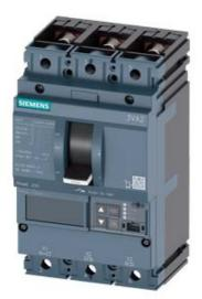
CIRCUIT BREAKER 3VA2 IEC FRAME 250 BREAKING CAPACITY CLASS C ICU=110KA @ 415 V 3POLE, LINE PROTECTION ETU850, LSI, IN=250A OVERLOAD PROTECTION IR=100A ...250A SHORT CIRCUIT PROTECTION ISD=0,6..10X IN, II=1,5..10X IN NEUTRAL PROTECTION OPTIONAL WITH EXT. CT,UPTO 160% BUSBAR CONNECTION
