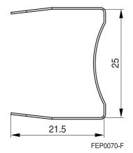
Dimensional tolerances +/-0,2 Dimensions in mm
