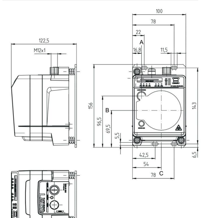
A Center axis of transmitter and alignment laser
