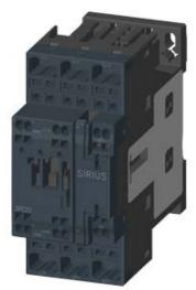
CONTACTOR, AC-3, 18.5KW/400V, 1NO+1NC, AC 230V 50/60HZ, 3-POLE, SZ S0 SPRING-LOADED TERMINAL
