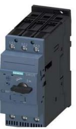
CIRCUIT BREAKER, SIZE S2, FOR MOTOR PROTECTION, CLASS 10, A-RELEASE 28...36A, N-RELEASE 520A, SCREW TERMINAL, INCREASED SWITCHING CAPACITY
