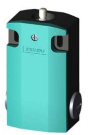
BASIC SWITCH FOR POSITION SWITCH 3SE5162, METAL ENCLOSURE XL,56MM WIDE DEVICE CONNECTION 3X(M20X1.5), IP66/IP67 2X (1NO/1NC)QUICK ACTION CONTACTS, WITHOUT ACTUATOR HEAD, WITH ENHANCED CORROSION PROTECTION
