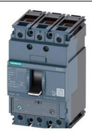
CIRCUIT BREAKER 3VA1 IEC FRAME 160 BREAKING CAPACITY CLASS S ICU=36KA @ 415 V 3-POLE, LINE PROTECTION TM240, ATAM, IN=100A OVERLOAD PROTECTION IR=70A ...100A SHORT CIRCUIT PROTECTION II=5...10 X IN CABLE CONNECTION
