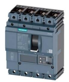
CIRCUIT BREAKER 3VA2 IEC FRAME 100 BREAKING CAPACITY CLASS H ICU=85KA @ 415 V 4POLE, LINE PROTECTION ETU550, LSI, IN=25A OVERLOAD PROTECTION IR=10A ...25A SHORT CIRCUIT PROTECTION ISD=0,6..10X IN, II=1,5..12X IN NEUTRAL PROTECTION ADJUSTABLE (OFF, UPTO 160%) BUSBAR CONNECTION
