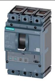
CIRCUIT BREAKER 3VA2 IEC FRAME 160 BREAKING CAPACITY CLASS M ICU=55KA @ 415 V 3POLE, LINE PROTECTION ETU330, LIG, IN=25A OVERLOAD PROTECTION IR=10A ...25A SHORT CIRCUIT PROTECTION II=1,5...12 X IN GROUNDFAULTPROTECTION IG=0,2... 1 X IN, TG=0,1/0,3MS CABLE CONNECTION
