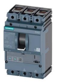
CIRCUIT BREAKER 3VA2 IEC FRAME 160 BREAKING CAPACITY CLASS C ICU=110KA @ 415 V 3POLE, LINE PROTECTION ETU320, LI, IN=63A OVERLOAD PROTECTION IR=25A ...63A SHORT CIRCUIT PROTECTION II=12 X IN CABLE CONNECTION
