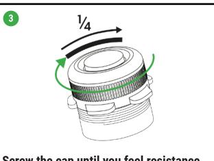
Screw the cap until you feel resistance. Then turn the cap an additional 1/4 of a turn. Do not tighten the cap too much, as it may be difficult to unscrew.
