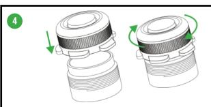
Place the cap back on the neck of the fuel can. Close the fuel can shut by screwing the cap clockwise.
