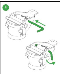
Insert the locking pin through the lever and rotate it 90 degrees.
