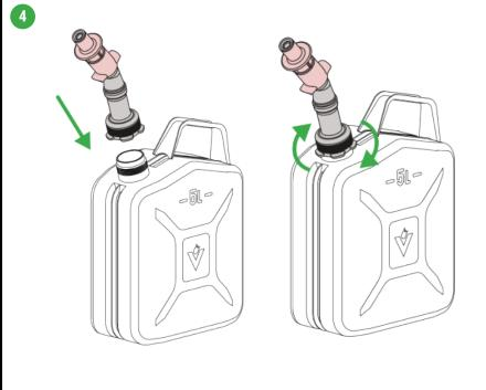
Screw the spout on by turning it clockwise until you feel resistance of the seal. Then turn the spout an additional 1/4 of a turn.
