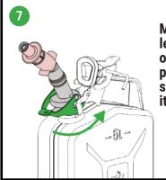
Move the arms of the lever into the cavities of the holder and push the lever of the spout down as far as it will go.
