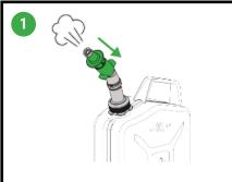
Press the tip of the spout to reduce the pressure of fuel vapour.
