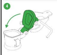
Push the lever forward until the lid completely covers the neck opening.
