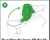
By pulling the lever, lift the lid up to open the neck opening.
