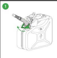
Pull back the lever of the fuel spout to remove the product from the fuel can.
