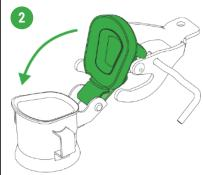
Push the lever forward until the lid completely covers the neck opening.
