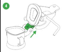
Before closing the fuel can lid, pull the lid with the hinge up by the lever.
