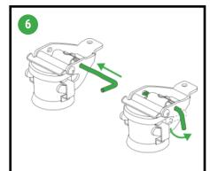
Insert the locking pin through the lever and rotate it 90 degrees.
