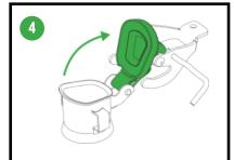
By pulling the lever, lift the lid up to open the neck opening.
