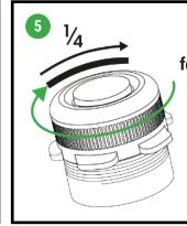
Screw the cap until you feel resistance. Then turn the cap an additional <sup>1</sup>/<sub>4</sub> of a turn. Do not tighten the cap too much, as it may be difficult to unscrew.
