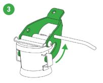
Lift the lever until the arms are fully released from the holder.
