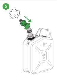
Before filling the fuel, press the tip of the spout to even out the fuel vapour pressure in the fuel can.
