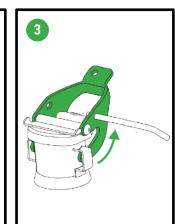
Lift the lever until the arms are fully released from the holder.
