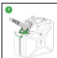
Move the arms of the lever into the cavities of the holder and push the lever of the spout down as far as it will
