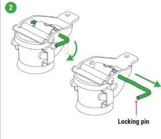
Turn the locking pin and pull it out of the lever as far as it will go.
