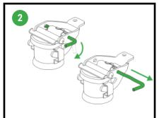
Turn the locking pin and pull it out of the lever as far as it will go.
