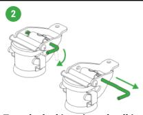
Turn the locking pin and pull it out of the lever as far as it will go.
