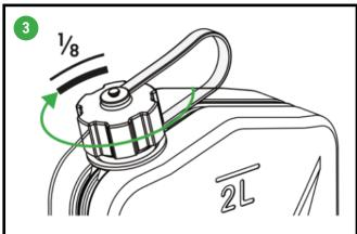
Screw the cap until you feel resistance. Then turn the cap an additional 1/8 of a turn. Do not tighten the cap too much, as it may be difficult to unscrew.
