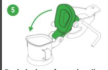
Push the lever forward until the lid completely covers the neck opening.
