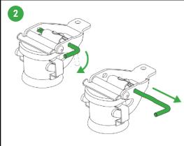
Turn the locking pin and pull it out of the lever as far as it will go.
