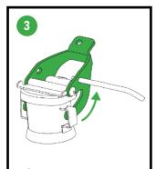
Lift the lever until the arms are fully released from the holder.
