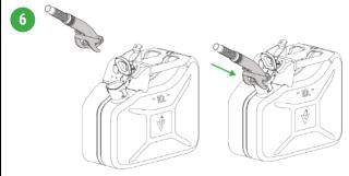
Place the fuel spout so it completely covers the neck opening of the fuel can.
