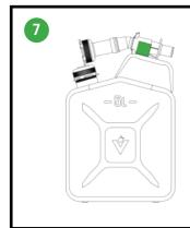
If the fuel can is equipped with a fuel spout holder, attach the spout to the holder for easier transportation.
