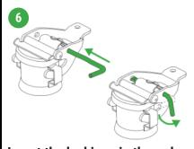
Insert the locking pin through the lever and rotate it 90 degrees.
