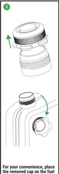
For your convenience, place the removed cap on the fuel can with the help of the incorporated magnet.
