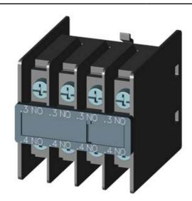
AUX.SWITCH BLOCK,FRONT,4NO, CURR.PATH: 1NO, 1NO, 1NO, 1NO, F. CONT. RELAYS A. MOTOR CONT., 3RT2 RING CABLE LUG CONNECTION .3 / .4,.3 / .4,.3 / .4,.3 / .4
