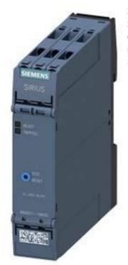
Thermistor motor prot. relay Standard evaluation unit 22.5 mm enclosure Screw terminals 2 CO contacts US = 24-240 V AC/DC Manual/Remote RESET with ATEX certification 2 LEDs (READY/TRIPPED) Galvanic separation Test/Reset button Open-circuit monitoring Short-circuit monitoring
