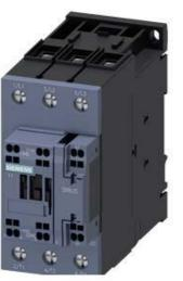
CONTACTOR,AC3:18.5KW/400V, 1NO+1NC, 110V AC 50HZ, 3-POLE, SIZE S2, SPRING-TYPE TERMINAL
