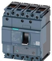
CIRCUIT BREAKER 3VA1 IEC FRAME 160 BREAKING CAPACITY CLASS H ICU=70KA @ 415 V 4-POLE, LINE PROTECTION TM240, ATAM, IN=125A OVERLOAD PROTECTION IR=87,5A ...125A SHORT CIRCUIT PROTECTION II=5...10 X IN NEUTRAL PROTECTION 100% CABLE CONNECTION
