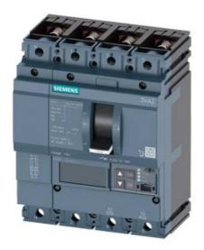
CIRCUIT BREAKER 3VA2 IEC FRAME 160 BREAKING CAPACITY CLASS C ICU=110KA @ 415 V 4POLE, LINE PROTECTION ETU550, LSI, IN=160A OVERLOAD PROTECTION IR=64A ...160A SHORT CIRCUIT PROTECTION ISD=0,6..10X IN, II=1,5..10X IN NEUTRAL PROTECTION ADJUSTABLE (OFF, UPTO 100%) BUSBAR CONNECTION
