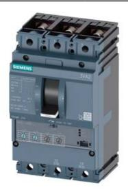
CIRCUIT BREAKER 3VA2 IEC FRAME 250 BREAKING CAPACITY CLASS M ICU=55KA @ 415 V 3POLE, LINE PROTECTION ETU330, LIG, IN=250A OVERLOAD PROTECTION IR=100A ...250A SHORT CIRCUIT PROTECTION II=1,5...10 X IN GROUNDFAULTPROTECTION IG=0,2... 1 X IN, TG=0,1/0,3MS BUSBAR CONNECTION
