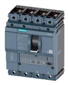
CIRCUIT BREAKER 3VA2 IEC FRAME 250 BREAKING CAPACITY CLASS L ICU=150KA @ 415 V 4POLE, LINE PROTECTION ETU350, LSI, IN=250A OVERLOAD PROTECTION IR=100A ...250A SHORT CIRCUIT PROTECTION ISD=1,5... 10 X IR, II=10 X IN NEUTRAL PROTECTION ADJUSTABLE(OFF,50%,100%) BUSBAR CONNECTION
