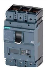
CIRCUIT BREAKER 3VA2 IEC FRAME 630 BREAKING CAPACITY CLASS C ICU=110KA @ 415 V 3-POLE, LINE PROTECTION ETU560, LSIG, IN=500A OVERLOAD PROTECTION IR=200A ...500A SHORT CIRCUIT PROTECTION ISD=0,6..10X IN, II=1,5..14X IN NEUTRAL PROTECTION OPTIONAL WITH EXT. CT;UPTO 160% GROUND-FAULT, SWITCHABLE IG=0,2... 1 X IN, TG=0,05-0,8MS BUSBAR CONNECTION
