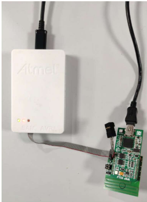
Figure 4-11. Connecting Programmer/Debugger with ATSAMR30M Sensor Board
