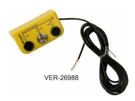
"The protection of ESDS [ESD sensitive item] is accomplished by providing a ground path to bring ESD protective materials and personnel to the same electrical potential. All conductor and dissipative items in the environment, including personnel, shall be bonded or electrically connected to a known ground or common connection point [Earth Bonding Point]." [CLC/TR 61340-5-2 User guide clause 4.4.1 Grounding/bonding systems Introduction]
