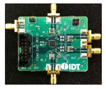
The F1240EVBI is a fully populated evaluation board which allows the customer to easily evaluate the F1240 Dual Intermediate Frequency Digital Variable Gain Amplifier. Attenuation may be set using either the F1240's parallel control input or its serial control input by setting Vmode to the appropriate value.
