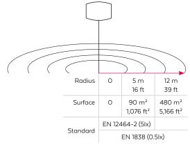
How to read the drawing: in a range of 12 m - 39 ft, being a surface of 480 m² - 5,166 ft², we guarantee a lighting in accordance with the EN 1838 standard.
