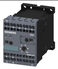
SOLID-STATE TIME-DELAY RELAY MULTI-FUNCTION, 8 FUNCTIONS 1 CHANGEOVER CONTACT AC/DC 24V, AC 200 TO 240V 0.05 S TO 100H WIDTH 45MM CAGE CLAMP
