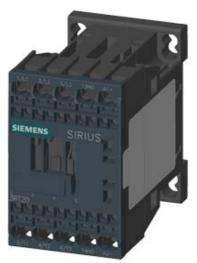
CONTACTOR, AC-3, 4KW/400V, 1NO, DC 24V, W. INTEGRATED DIODE 3-POLE, SZ S00 SPRING-LOADED TERMINAL
