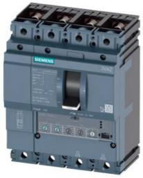
CIRCUIT BREAKER 3VA2 IEC FRAME 100 BREAKING CAPACITY CLASS M ICU=55KA @ 415 V 4POLE, LINE PROTECTION ETU350, LSI, IN=25A OVERLOAD PROTECTION IR=10A ...25A SHORT CIRCUIT PROTECTION ISD=1,5... 10 X IR, II=12 X IN NEUTRAL PROTECTION ADJUSTABLE(OFF,100%) BUSBAR CONNECTION
