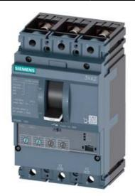
CIRCUIT BREAKER 3VA2 IEC FRAME 160 BREAKING CAPACITY CLASS M ICU=55KA @ 415 V 3POLE, LINE PROTECTION ETU330, LIG, IN=40A OVERLOAD PROTECTION IR=16A ...40A SHORT CIRCUIT PROTECTION II=1,5...12 X IN GROUNDFAULTPROTECTION IG=0,2... 1 X IN, TG=0,1/0,3MS BUSBAR CONNECTION
