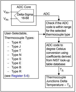
**FIGURE 5-3:** Thermocouple Hot-Junction Register  $(T_{\Delta})$  Block Diagram.
