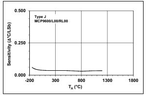
**FIGURE 2-5:** Temperature Sensitivity with 18-Bit Resolution, Type J.
