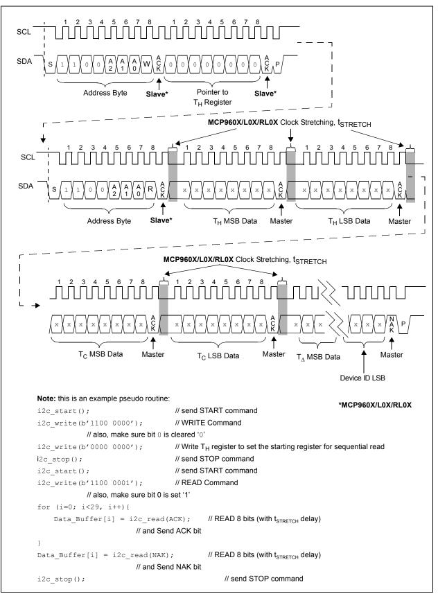
**FIGURE 4-6:** Timing Diagram to Sequential Read All Registers Starting from T<sub>H</sub> Register.
