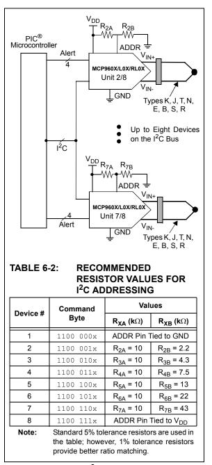
**FIGURE 6-4:** I<sup>2</sup>C Address Selection Implementation.
