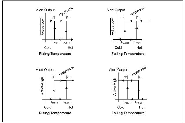
FIGURE 5-10: Graphical Description of Alert Output Hysteresis Direction.
