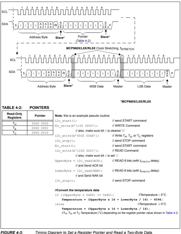
Timing Diagram to Set a Register Pointer and Read a Two-Byte Data.
