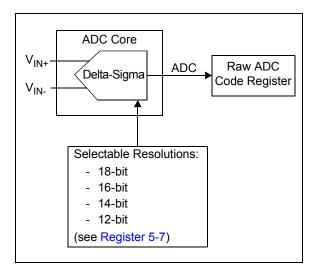
FIGURE 5-5: Delta-Sigma Analog-to-Digital Converter, ADC Core Block Diagram.
