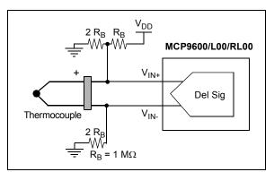
**FIGURE 6-6:** Adding Open-Circuit Detection Resistors (MCP9600/L00/RL00).
