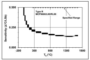
**FIGURE 2-11:** Temperature Sensitivity with 18-Bit Resolution, Type R.
