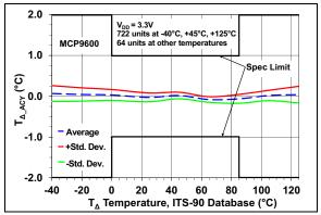
FIGURE 2-20: Cold-Junction Sensor Temperature Accuracy.
