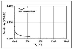
**FIGURE 2-16:** Temperature Sensitivity with 18-Bit Resolution, Type T.
