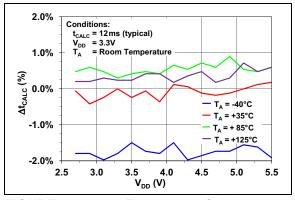
**FIGURE 2-30:** Temperature Calculation Duration,  $t_{CALC}$  Change Across  $V_{DD}$ .
