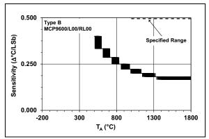
**FIGURE 2-17:** Temperature Sensitivity with 18-Bit Resolution, Type B.
