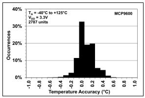
**FIGURE 2-23:** Cold-Junction Sensor Temperature Accuracy Distribution.
