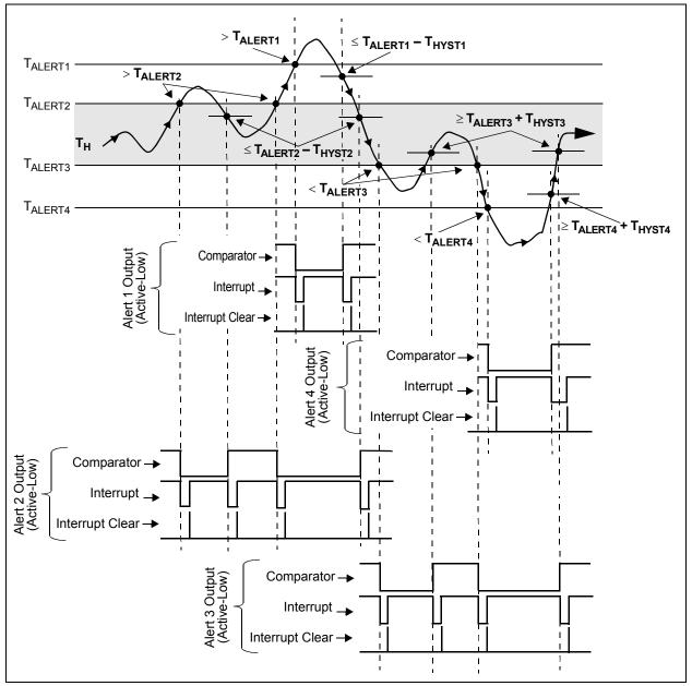
FIGURE 5-9: Alert Limits Boundary Conditions and Output Characteristics when Set to Detect T<sub>H</sub>.
