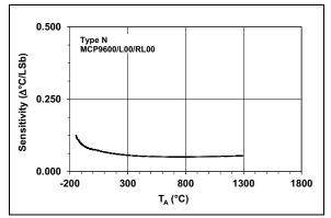
**FIGURE 2-6:** Temperature Sensitivity with 18-Bit Resolution, Type N.
