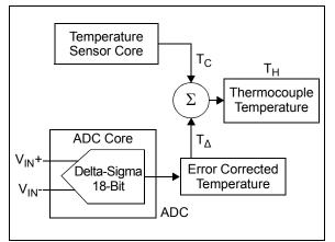
FIGURE 5-2: Thermocouple Temperature Register Block Diagram.
