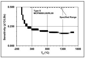
**FIGURE 2-10:** Temperature Sensitivity with 18-Bit Resolution, Type S.
