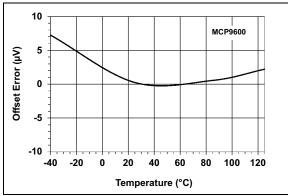
**FIGURE 2-15:** Input Offset Error Voltage  $(V_{IN+}, V_{IN-})$ .
