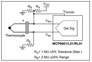
**FIGURE 6-7:** Adding Open-Circuit Detection Resistors (MCP9601/L01/RL01).
