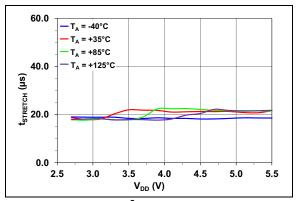
**FIGURE 2-29:** I<sup>2</sup>C Interface Clock Stretch Duration, t<sub>STRETCH</sub> Across V<sub>DD</sub>.
