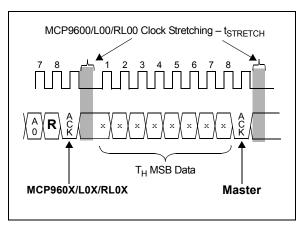
FIGURE 4-2: Clock Stretching.
