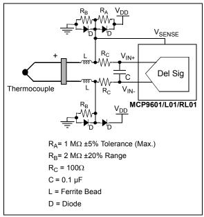
FIGURE 6-12: Adding Ferrite Beads (MCP9601/L01/RL01).
