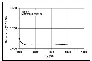
**FIGURE 2-4:** Temperature Sensitivity with 18-Bit Resolution, Type K.
