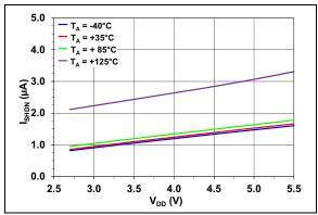
**FIGURE 2-27:** Shutdown Current, I<sub>SHDN</sub> Across V<sub>DD</sub>.
