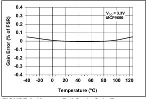
FIGURE 2-18: Full-Scale Gain Error.
