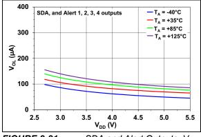
**FIGURE 2-21:** SDA and Alert Outputs, V<sub>OL</sub> Across V<sub>DD</sub>.
