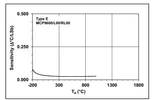
**FIGURE 2-12:** Temperature Sensitivity with 18-Bit Resolution, Type E.
