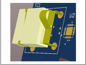
FIGURE 6-2: Recommended Component Placement.
