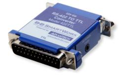
Model BB-422TTL converts RS-422 or EIA-530 signals to 5V TTL at data rates up to 115.2 kbps. Two channels are used to convert RS-422 to TTL and two channels are used to convert TTL to RS-422.
