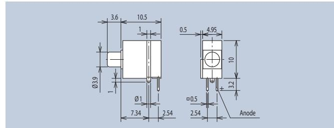
These components with lateral fins and grooves, which interlock when being stacked, guarantee appropriate stabilization on the printed circuit board. With an integrated protective resistor this component is suitable for low-current applications, too. Various operating voltages are available.
