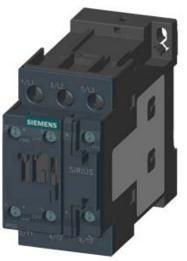
CONTACTOR, AC-3, 7.5KW/400V, 1NO+1NC, AC(50-60HZ)/DC ACTUAT. AC/DC 200...280V, 3-POLE, SZ S0 SCREW TERMINAL
