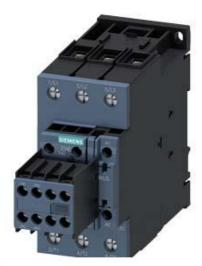
CONTACTOR,AC3:22KW/400V, 2NO+2NC, 48 - 80V AC/DC, WITH VARISTOR, 3-POLE, SIZE S2, SCREW TERMINAL
