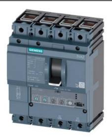
CIRCUIT BREAKER 3VA2 IEC FRAME 100 BREAKING CAPACITY CLASS H ICU=85KA @ 415 V 4POLE, LINE PROTECTION ETU330, LIG, IN=25A OVERLOAD PROTECTION IR=10A ...25A SHORT CIRCUIT PROTECTION II=1,5...12 X IN NEUTRAL PROTECTION ADJUSTABLE(OFF,100%) GROUNDFAULTPROTECTION IG=0,2... 1 X IN, TG=0,1/0,3MS CABLE CONNECTION
