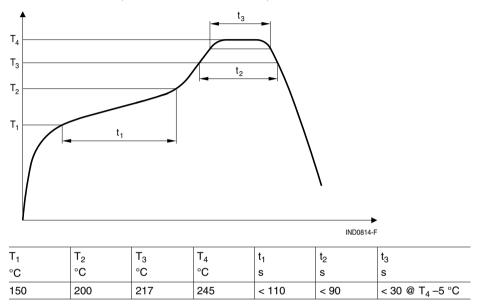
Time from +25 °C to  $T_4$ : max 300 s Max. numbers of reflow cycles: 3
