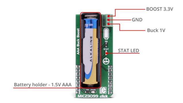
Note: The MIC23099 is not a battery charger and it needs a battery to work properly. The battery is not included.
