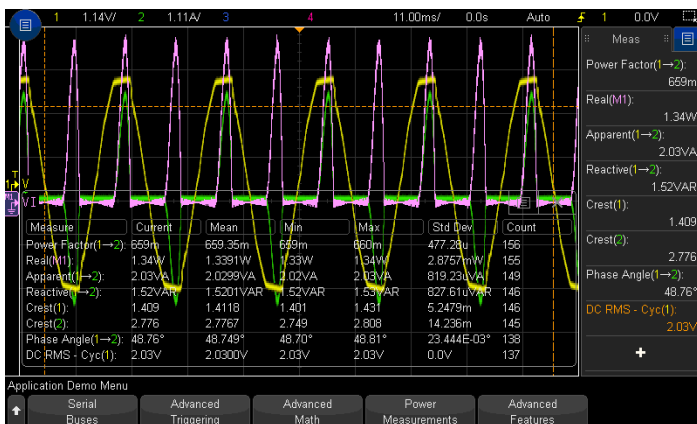
Figure 29: Integrated power measurements make quick work of analyzing power producing and power consuming devices.
