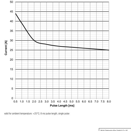
Typical Peak Current vs. Pulse Length Characteristics:
