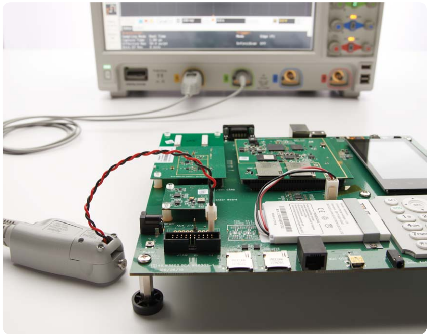
Figure 1. Agilent's ultra sensitive N2820A/N2821A current probes (with resolution as low as 50 \mu\text{A} ) excel at measuring for small current levels typically found in battery powered devices.
