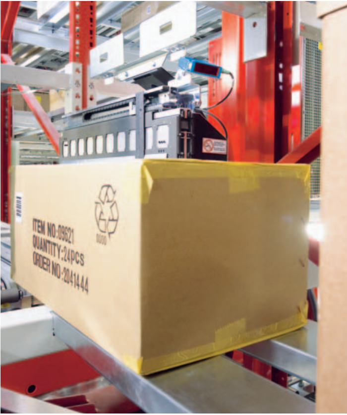
◀ The WT34 photoelectric proximity switch stands out for its large scanning distance with regard to checking whether second or backward storage bays are occupied.
