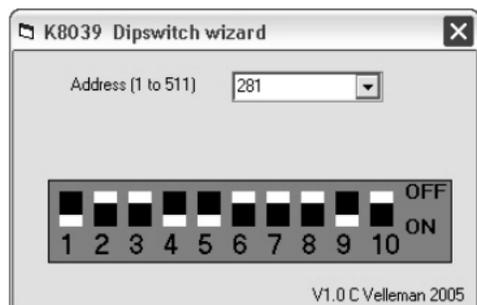
4. Switch 10 of the SW1 to ON when using the K8039 as sole connected DMX device or when it is the last connected device in the series.
